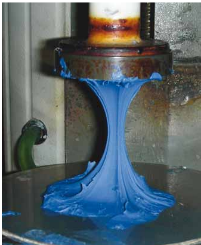
Figure 2. Viscotaq is a smart coating with viscous-elastic and self-healing properties.
